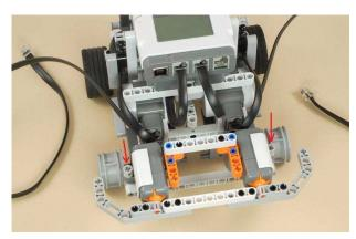
The touch sensor is a simple binary switch whose state is either 0 or 1 depending on whether it is pressed. Mount two touch sensors onto the front of your robot with a simple bumper mechanism which might be similar to the one in the picture above. Adding the long blocks to the front of the touch sensors creates a bumper which should effectively be able to detect when the robot collides with an obstacle when driving forwards, causing either or both of the touch sensors to be activated.
